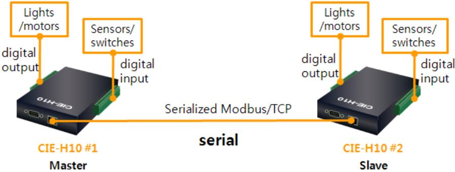
Figure 1-4 serial switch
