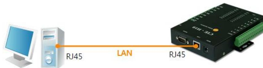
Figure 2-1 the connection between CIE-H10 and a PC
