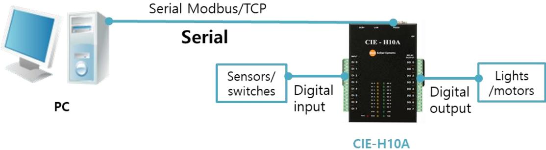
Figure 1-2 serialized Modbus/TCP
