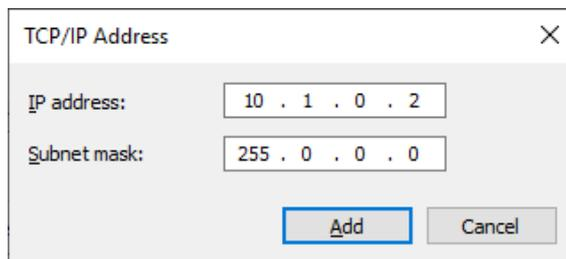
Figure 2-2 adding / changing an IP address
