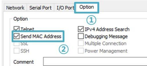
Figure 8-2 setting of Sending MAC Address function
