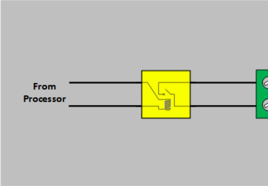
Figure 1-8 a circuit of the output port
