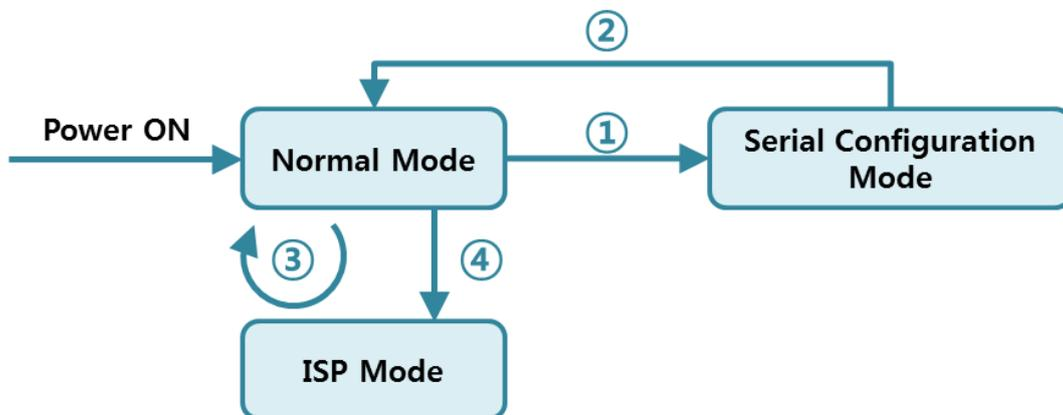
Figure 4-1 How to enter into each mode
