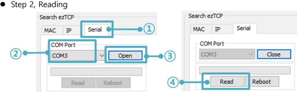
Figure 3-4 reading procedure via serial
