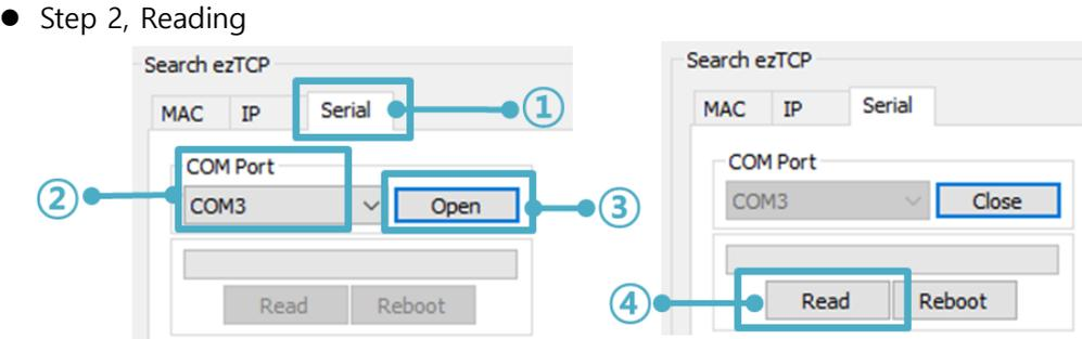
Figure 3-4 reading procedure via serial
