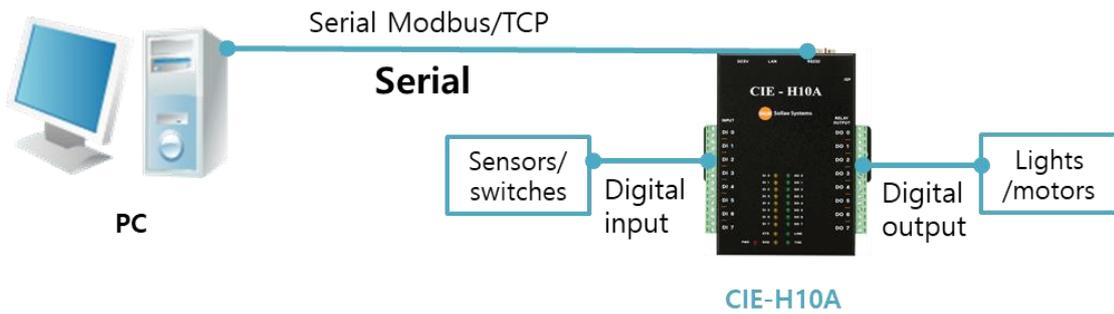
Figure 1-2 serialized Modbus/TCP
