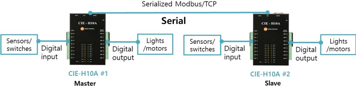
Figure 1-4 serial switch
