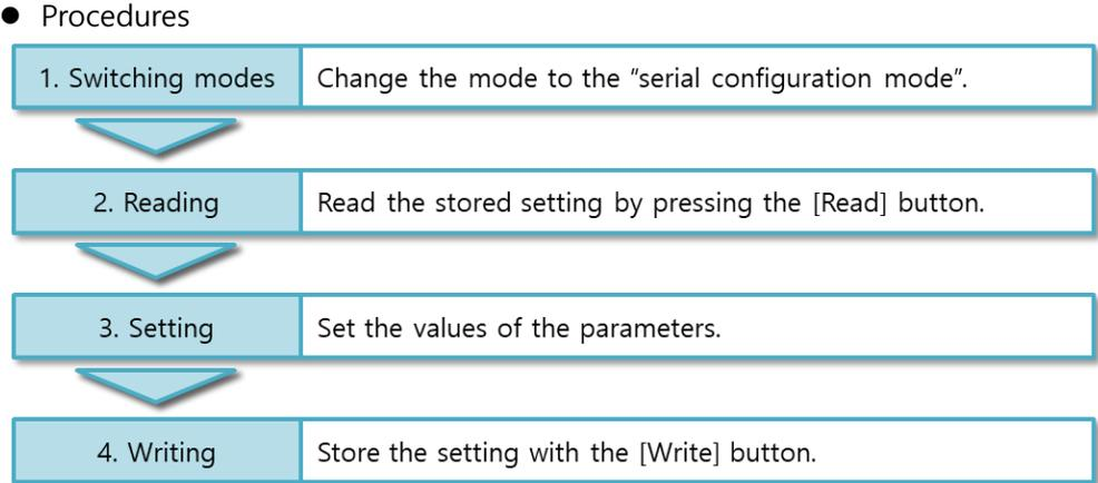
Figure 3-3 procedures for configuration via serial port
