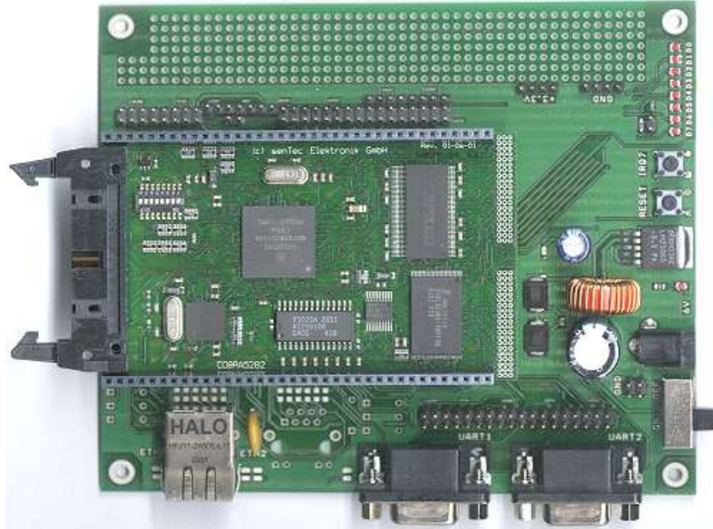
Figure 3 COBRA5282 Module connected to the Carrier Board
