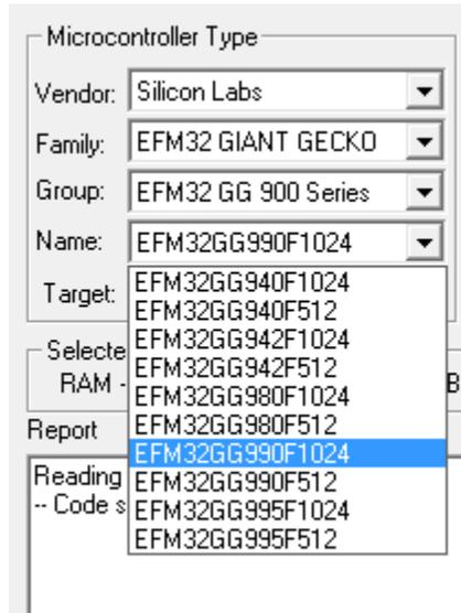
Figure 4.2: The MCU type can be selected here.
