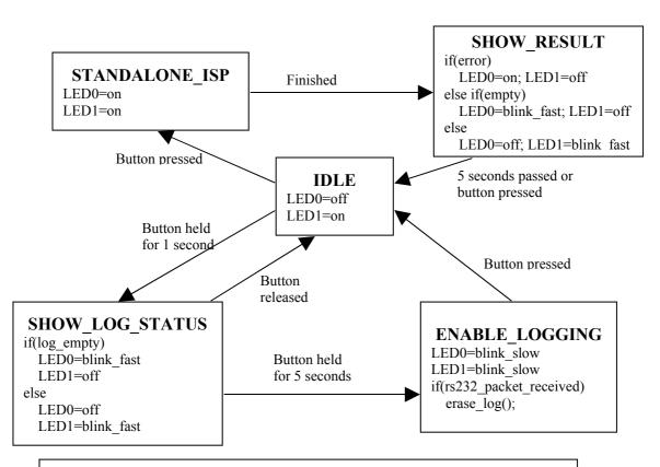
NOTE: LED0 is **RED**, and LED1 is **GREEN**. If both are on, the result is **Yellow** glow.
