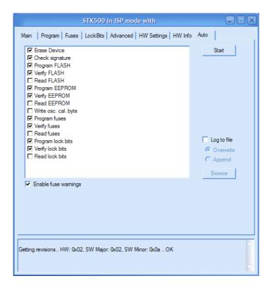
Select the operations that should be performed and hold the programmer button for 5 seconds to activate command logging. Then hit the "Start" button to initiate a programming operation. After "Auto" operation finishes successfully, turn off command logging.
