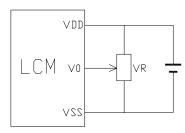
$V_{DD\sim}V_0$ : LCD Driving voltage VR:  $10k\sim20k$
