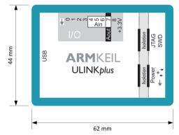
**ULINK***plus* is a universal debug and trace adapter that enables test automation, software optimization for ultra-low-power applications, and isolation for debugging sensitive hardware systems. The compact enclosure allows usage in harsh environments and provides standard target connectors for JTAG, power measurement, and general purpose I/O.
