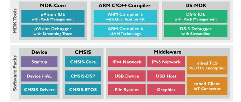
MDK-Core offers leading support for over 3,750 Cortex-M based devices including the new ARM Cortex-M23/M33 cores. The µVision debugger includes event recorder and component viewer to show run-time behavior of software components. Together with the ULINK*pro*™ debug adapter, it offers full instruction trace and complete code coverage information.
