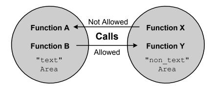
The above diagram shows a scenario that is problematic. Code areas created with the AREA directive, using a name other than text, are not compressed or fixed up following compression. If Function Y calls Function B, there is the potential that the location of Function B will be changed by the Code Compressor. The call or jump generated in the code for Function Y will go to the wrong location.
